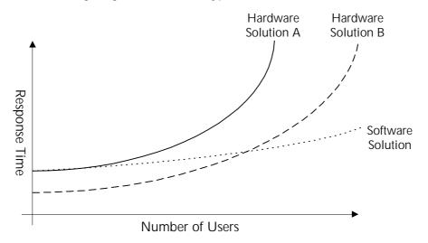
We see a hardware solution A reaching a *thrashing point* at which no useful work gets done any longer. By installing a hardware solution B that is twice as fast, we get an improvement in performance, but we still reach a thrashing point fairly quickly because we have not resolved the basic inefficiencies of the software. With a software solution we can flatten the curve and prevent thrashing even with high numbers of users.
