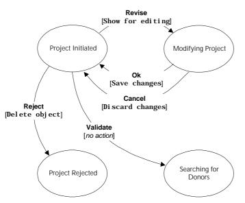
Here the methods are Revise, Ok, Cancel, Validate, and Reject. The states are circled, and the actions are indicated [like this]. Note the difference between the Reject method, the [delete object] action, and the 'Project Rejected' state.
