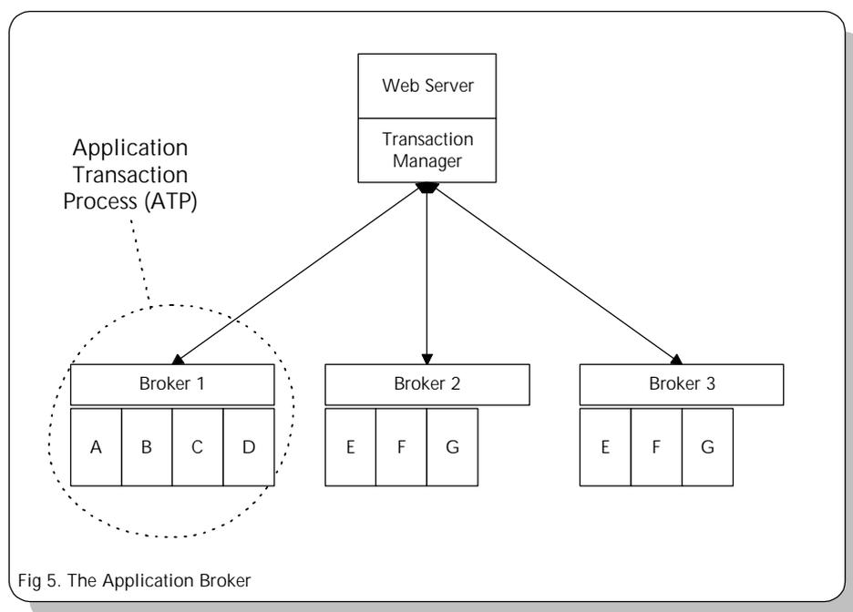
The WTP manager is responsible for starting, monitoring, and halting ATP processes as required. One WTP manager (there may be several active on a particular host machine) is responsible for handling a set of WTP applications. For instance, one WTP manager could handle the development, test, and production versions of a client control application. Each of these applications can be stopped and started independently.
